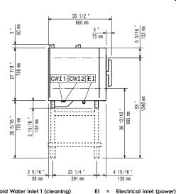
Cold Water inlet 1 (cleaning) CWII Cold Water Inlet 2 (steam CWI2
